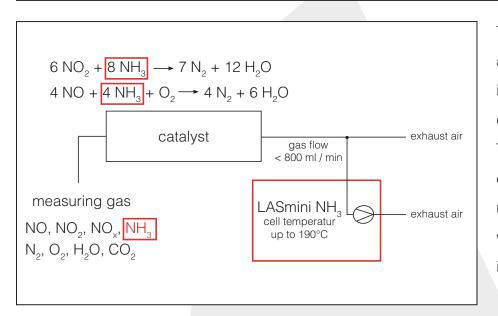
The exact measurement of ammonia  $(NH_3)$  is of particular importance in the development of catalysts (SCR) or their sensors. The coordination of catalyst efficiency and consumables is reflected in the ammonia slip, which is continuously determined in the hot measuring gas.
