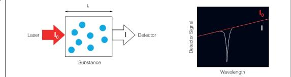
The measured spectrum and the model for the instrument function are compared with the HITRAN database containing the theoretical absorption spectrum of  $NH_3$ . The analysis algorithm continuously verifies the absence of divergences and ensures a correct measurement.
